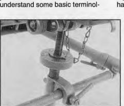
The M2/M122 tripod's traversing bar has an engraved scale to assist in measuring or establishing horizontal angles. The elevating handwheel assembly has a mil click device built into it. Note that the 50-mil scale engraved on the upper surface of the handwheel is divided into 5-mil major graduations and 1-mil subdivisions.
